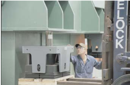
An isolator being lifted into place under a press foot.
