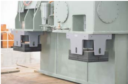
The isolators are attached to the press feet.
